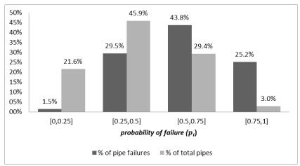
Fig 5 Percentage of prevented failures and percentage of total pipes for different ranges of  $p_i$  (figure created with MSOffice)
