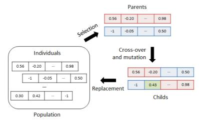
Fig 1 A visual illustration of the designed genetic algorithm (figure created with MSOffice)
