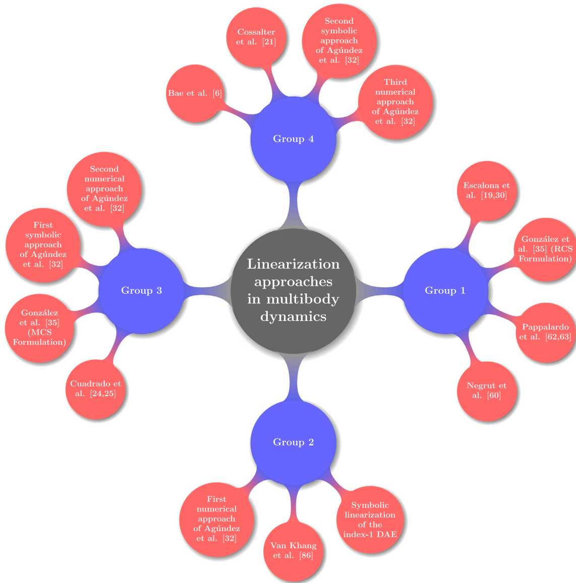
Fig. 1. Linearization approaches in multibody dynamics considered in this work, classified into four groups. Group 1 (Section 3.1) encompasses the procedures based on the linearization of the index-3 DAE system, using a redundant set of coordinates. The linearization approaches considered in Group 1 are the procedure by Escalona et al. [5,6], the Redundant Coordinate Set (RCS) approach by González et al. [7], the procedure by Negrut et al. [4] and the linearization approach by Pappalardo et al. [8,9]. Group 2 (Section 3.2) includes those procedures based on the linearization of the index-1 DAE system, using a redundant set of coordinates. The symbolic linearization of the index-1 DAE system, the approach by Van Khang et al. [12] and the first numerical procedure by Agúndez et al. [13] are considered in Group 2. Group 3 (Section 3.3) comprises linearization procedures based on coordinate partitioning in terms of independent and dependent coordinates. The procedures by Cuadrado et al. [15,16], the Minimal Coordinate Set (MCS) approach by González et al. [7], and the first symbolic and second numerical procedures by Agúndez et al. [13] are included. Lastly, Group 4 (Section 3.4) includes linearization procedures, based on a coordinate partition in terms of independent and dependent coordinates, with holonomic constraints elimination. The procedure by Bae et al. [26], the approach by Cossalter et al. [27] and the second symbolic and third numerical approaches by Agúndez et al. [13] are considered in Group 4.
