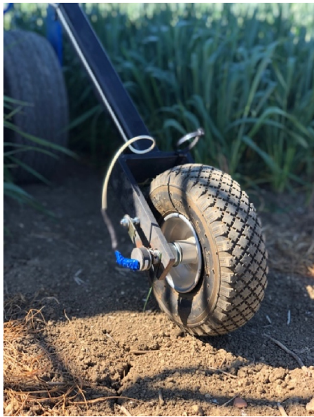
Fig. 4. Ground wheel odometry system attached to the HTPP chassis.
