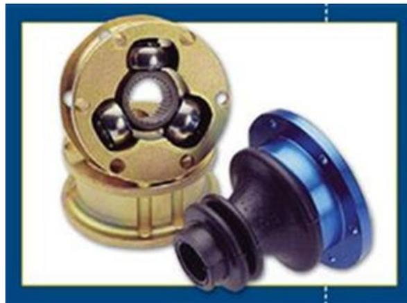
Figura 4-49. Junta GKN GI3300i
