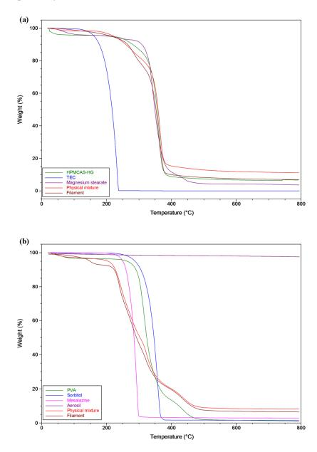
**Figure 4.** TGA thermograms of (**a**) HPMCAS-HG, TEC, magnesium stearate, and the corresponding physical mixture and extruded filament, (**b**) PVA, sorbitol, mesalazine, Aerosil<sup>®</sup>, and the corresponding physical mixture and extruded filament.
