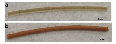
**Figure 2.** Digital pictures of (**a**) extruded HPMCAS-HG filament, (**b**) extruded drug-loaded PVA filament.
