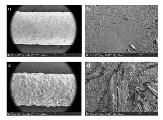
**Figure 6.** SEM microphotographs of (**a**) surface of HPMCAS-HG filament ( $50 \times$ ); (**b**) cross-section of HPMCAS-HG filament ( $500 \times$ ); (**c**) surface of drug-loaded PVA filament ( $50 \times$ ); (**d**) cross-section of drug-loaded PVA filament ( $500 \times$ ).
