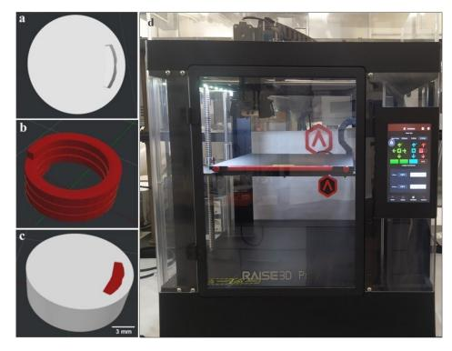
**Figure 1.** Digital designs (IdeaMaker software version 3.1.7) of (**a**) cylindrical HPMCAS-based external compartment (top view), (**b**) drug-loaded PVA-based internal compartment (spiral shape), (**c**) bicompartmental device for FDM printing using a Pro2 Dual Extruder Raise3D printer (**d**).
