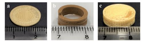
**Figure 8.** Pictures of 3D-printed devices: (**a**) cylindrical HPMCAS-based external compartment (top view), (**b**) drug-loaded PVA-based internal compartment (spiral shape), (**c**) bicompartmental device.
