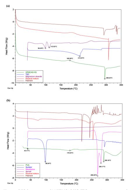
**Figure 3.** DSC thermograms of (**a**) HPMCAS-HG, TEC, magnesium stearate, and the corresponding physical mixture and extruded filament, (**b**) PVA, sorbitol, mesalazine, Aerosil<sup>®</sup>, and the corresponding physical mixture and extruded filament.
