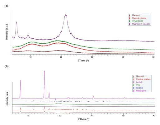
**Figure 5.** X-ray powder diffractograms of (**a**) HPMCAS-HG, magnesium stearate, and the corresponding physical mixture and extruded filament, (**b**) PVA, sorbitol, mesalazine, Aerosil<sup>®</sup>, and the corresponding physical mixture and extruded filament.
