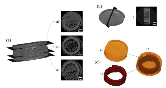
Figure 10.  $X\mu$ CT images of the 3D-printed bicompartmental device: (a) horizontal cross-section slices ((a1-a3), bottom to top), (b) vertical cross-section slice, (c) image segmentation and reconstruction of the 3D-printed bicompartmental device architecture ((c1)—inner compartment, (c2)—outer compartment, (c3)—whole structure).
