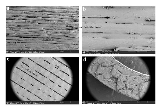
**Figure 9.** SEM microphotographs of (**a**,**b**) HPMCAS-based external compartment of the 3D-printed device (radial view,  $100 \times$  and  $500 \times$ ); (**c**) HPMCAS-based external compartment of the 3D-printed device (axial view,  $50 \times$ ); (**d**) PVA-based internal compartment of the 3D-printed device (axial view,  $50 \times$ ).
