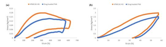
**Figure 7.** Representative stress–strain curves of three-point bending (3PB) (**a**) and stiffness (**b**) tests of HPMCAS-HG and drug-loaded PVA filaments.
