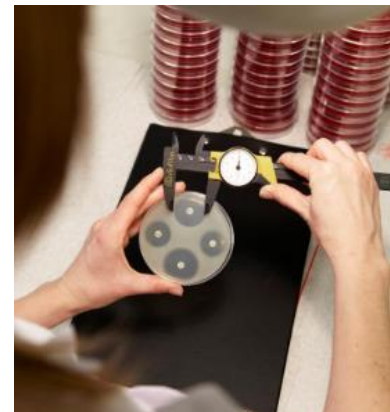
Figure 17. Antibiogram reading by measuring the diameter of the inhibition halo with the disc-diffusion technique 200 .
