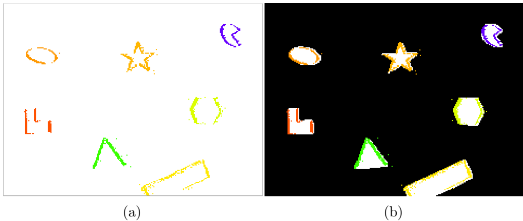
Figure 2.6: (a) Clusters of events obtained by using the proposed method, and (b) their equivalent representation after being rendered over the mask I_M . The color of each event sample (i.e., colored pixels) indicates the cluster identifier.
