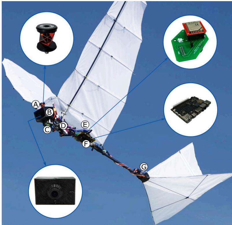
Figure 6.6: Distribution of the perception hardware on the GRIFFIN Eye-Bird in an experimental scenario: (A) Leica GRZ101 MiniPrism, (B) DAVIS346 camera, (C) battery, (D) the flapping mechanism, (E) VectorNav VN-200 IMU, (F) Khadas VIM3 board, and (G) tail servos.
