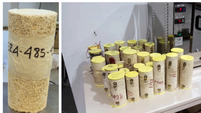
Fig. 2. Cylindrical specimens extracted from columns and walls of Santiago Church (Jerez de la Frontera, Cadiz - Spain).
