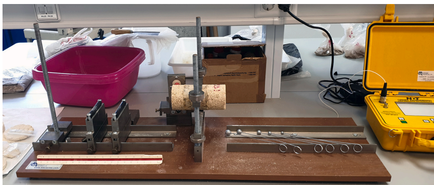
Fig. 4. Test performed to obtain the dynamic elastic modulus.
