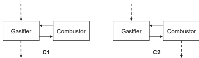
Fig. 2. Configurations for the integration of the solids heat carrier into the SDFBG system (dashed arrows represent the circulation from/to the solar loop; solid arrows defined as in Fig. 1(a)).
