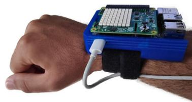
**Fig. 1** Electronic wearable device placed at the wrist of the player. It is based on Raspberry pi 4 with Sense HAT module that incorporates an IMU sensor
