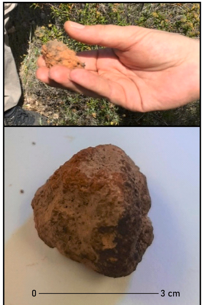
Fig. 8. Evidence de carbonization in clay nodules.
