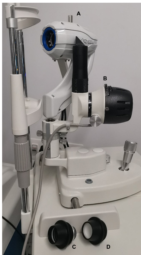
FIGURE 1 Ocular Surface Analyzer (OSA) device fit in a slit lamp tonometer hall. (A) OSA measurement head device. (B) Slit lamp illumination system. (C) Placido grid measurement cone. (D) Plain measurement cone.
