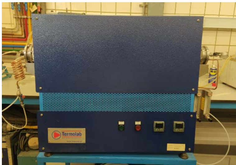
Figure 3. 14 - Tubular furnace (TermoLab)
