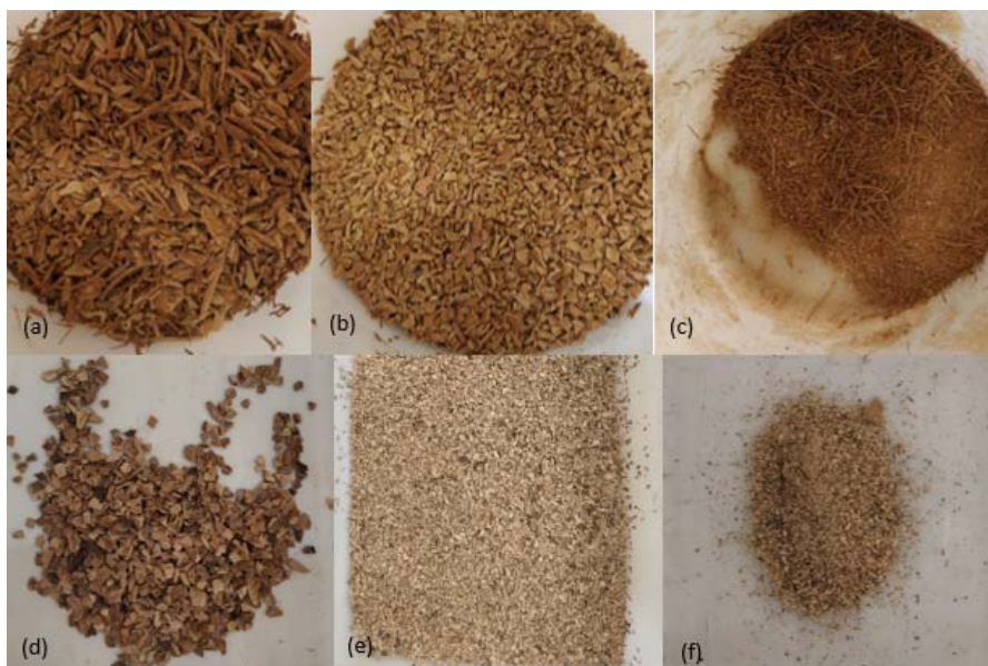
Figure 3. 6 - (a) Almond shells [ >2,83\text{mm} ]; (b) Almond shells [ 1-2,83\text{mm} ]; (c) Almond shells [ <1\text{mm} ]; (d) Walnut shells [ >2,83\text{mm} ]; (e) Walnut shells [ 1-2.83\text{mm} ]; (f) Walnut shells [ <1\text{mm} ]
