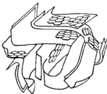
Figure 2. 6 - Schematic representation of microstructure of activated carbon (Luka et al., 2018)
