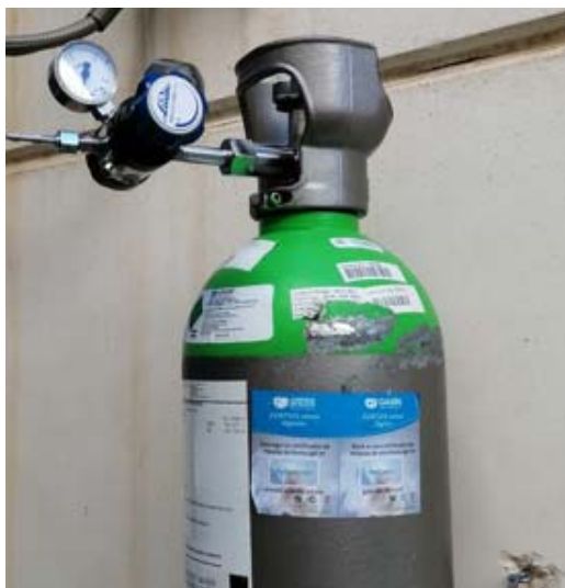
Figure 3. 17 - Simulated biogas bottle, with pressure reducer and pressure gauges
