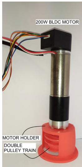
(a) Actuation system. Motor, motor holder and double pulley
