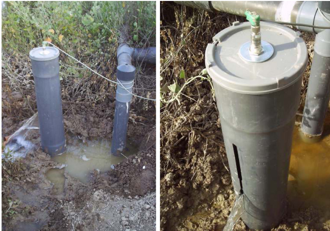
Fig. 2 – Photograph of one of the flow meters operating in field conditions.
