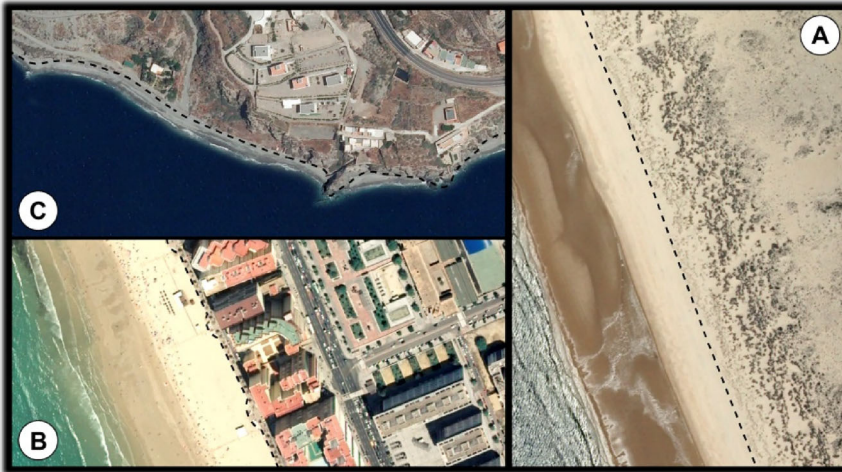
Figure 2. The proxy used to discriminate the contact between the backshore and the foredune (A), infrastructure (B) or cliff (C), depending on the coastal section. All examples are from the Andalusian coast.
