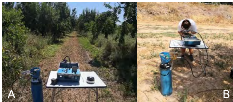
Figure 2.5 (A). Scholander camera. (B). Measurement with the Scholander camera in the field.
