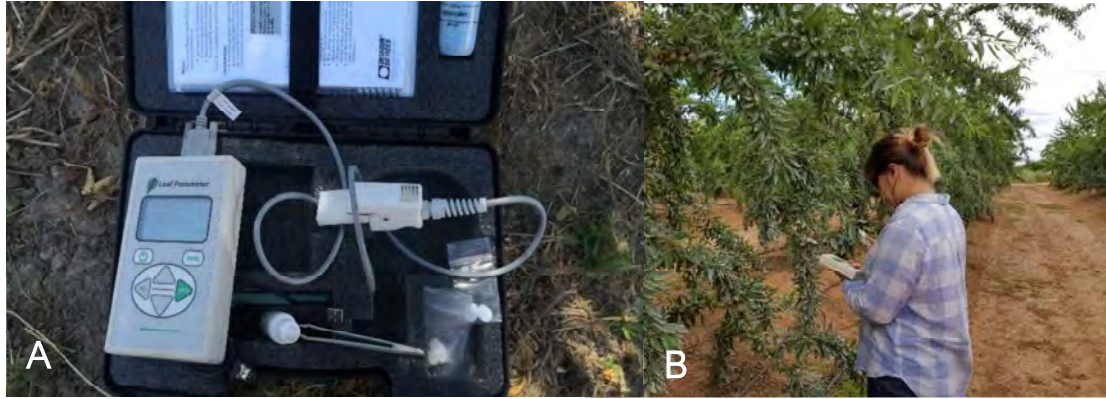
Figure 2.6 (A). Porometer SC-1. (B). Field measurement with the porometer SC-1.
