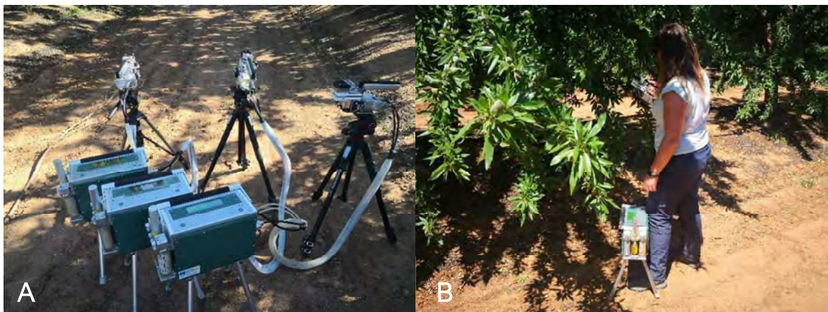
Figure 2.9 (A). Three LI-6400 portable photosynthesis system (LI-COR, Lincoln, NE, USA). (B). Field measurement with LI-6400.
