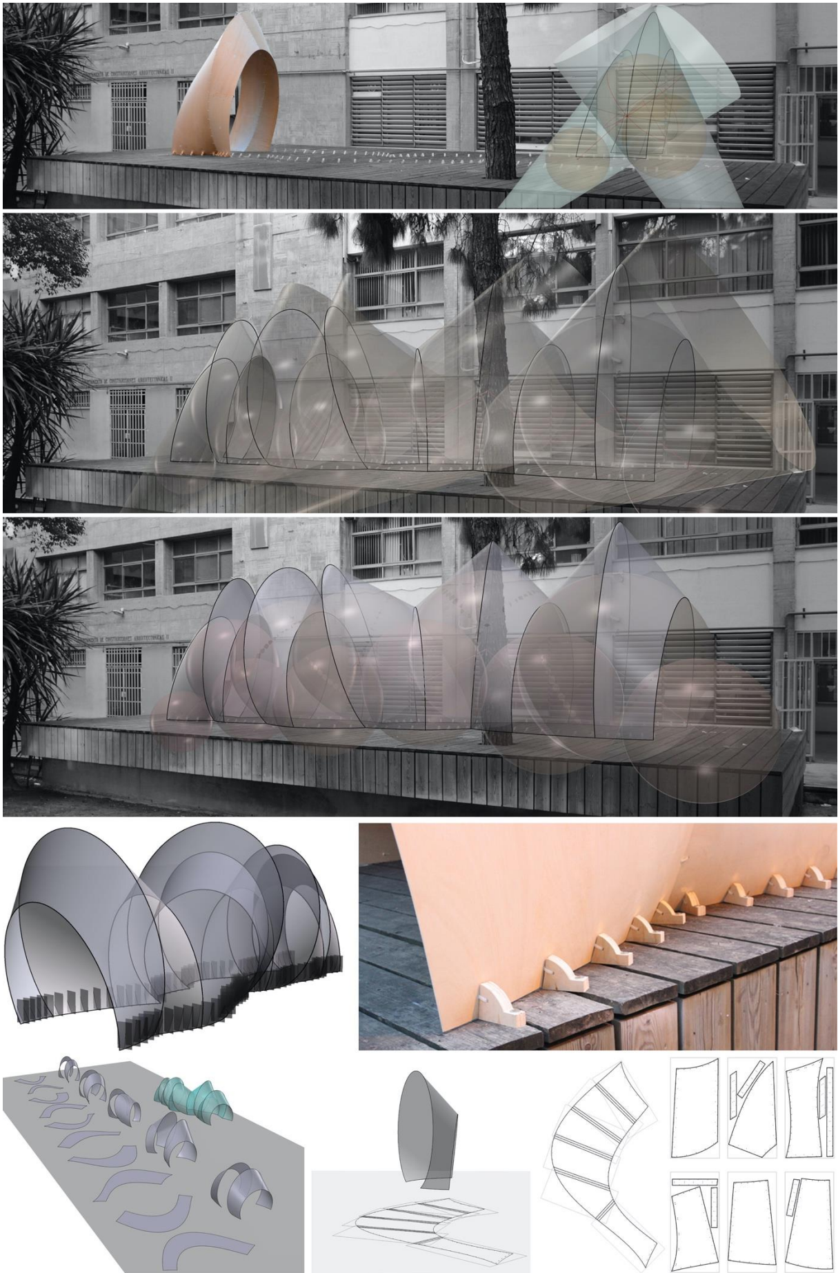
Fig. 6. Top three rows: composition of the installation on the site. Middle row: automation to determine the shape of the wedges. Bottom row: Development of the surfaces and graphic documentation for digital fabrication.
