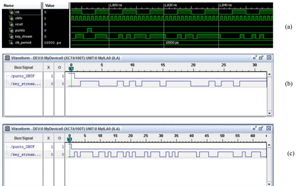
Fig. 3. Performance screenshots: (a) functional, (b) correct operation observed with Chipscope at 500 MHz, (c) incorrect operation observed with Chipscope at 600 MHz
