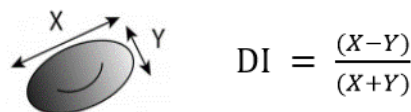
Figure 3.21 Schematic representation of a deformed particle and definition of the deformation index (DI).
