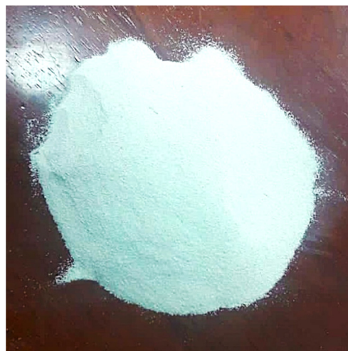
Figure 1. Bioceramics powder used as an aggregate for the development of the new mortars.
