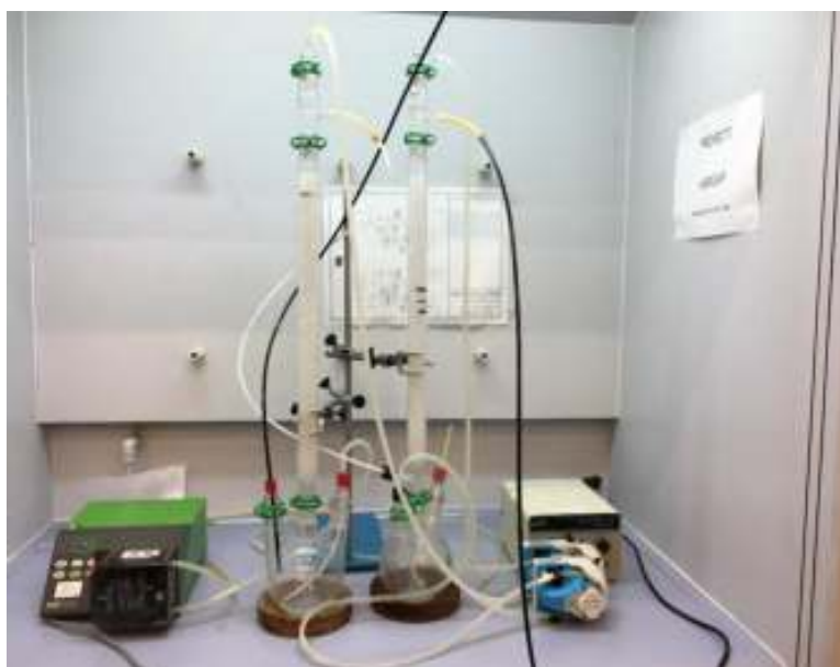
Figure 7.8. Absorption tower used for NH 3 solvent characterization.
