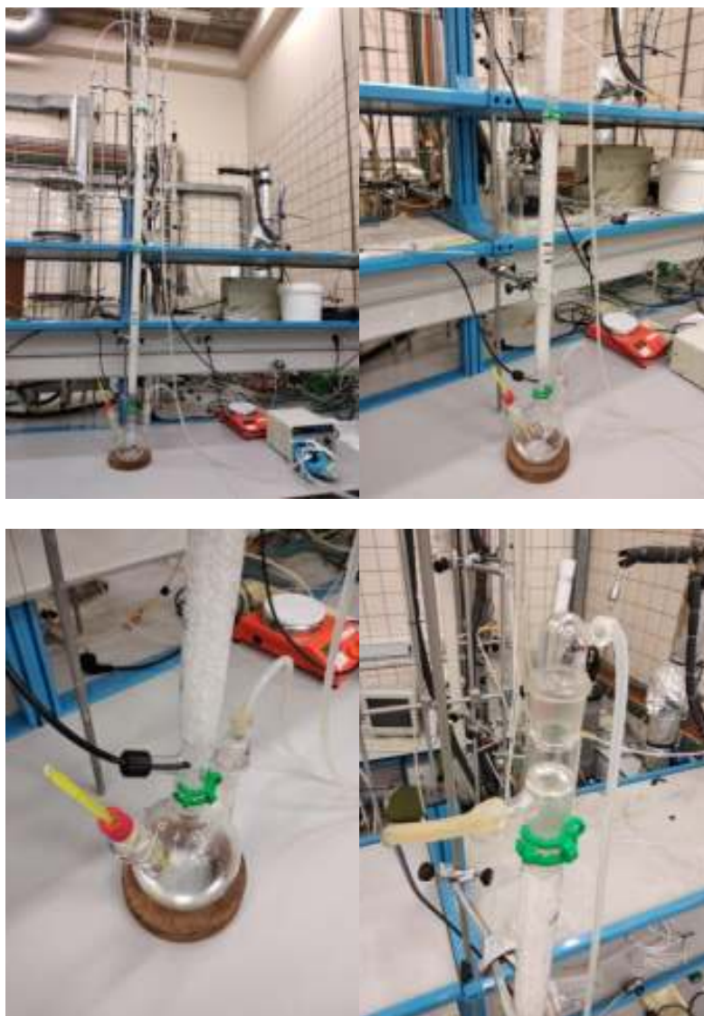
Figure 7.7. Absorption tower used for NaOH, KOH and MEA solvents characterization.
