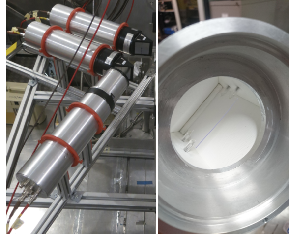
Figure 4. Left: structure of the triple-stage RPT-PTB: three plastic scintillators. Right: detail of the interior of the cover for the \Delta\text{E} detectors with a diffuse white reflector to reduce the inhomogeneity of the light collection.
