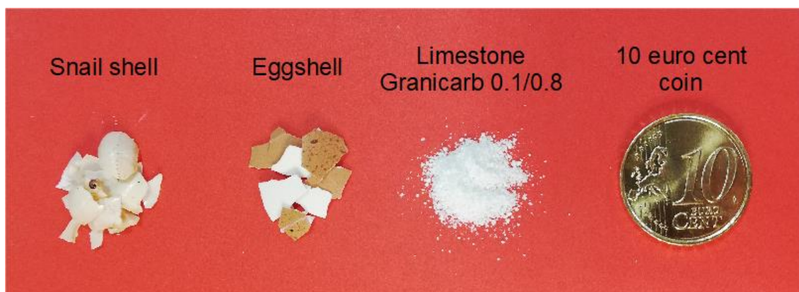
FIG. 1: Photograph of the untreated shells and the sample of limestone used in this work.
