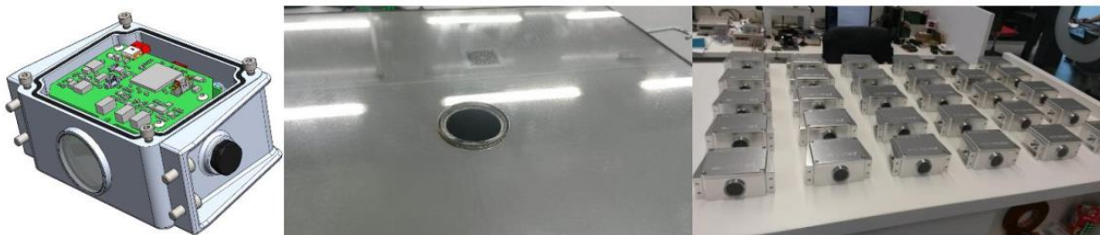
Figure 6-9 SMARTMIRROR black box configuration. Left: Sensor 3D design. Centre: Sensor integrated into a mirror. Right: 30 sensors manufactured and assembled; ready to be integrated into the mirrors at the site (La Africana) (Calvo et al., 2020)
