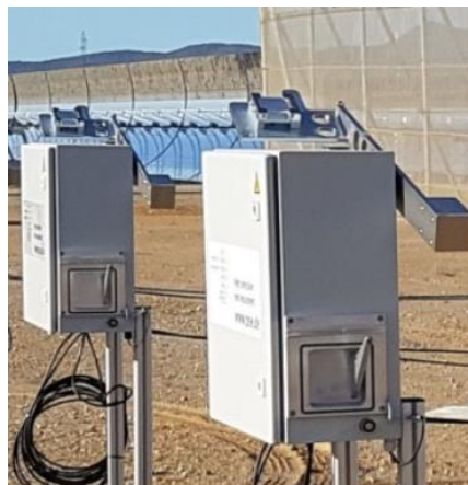
Figure 6-6 AVUS instrument prototypes for automated in-situ soiling rates and cleanliness (Heimsath, 2018)
