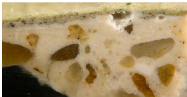
Figure 7: The presence of a high quantity of sand typical of murals at Vremski Britof and Famlje.
