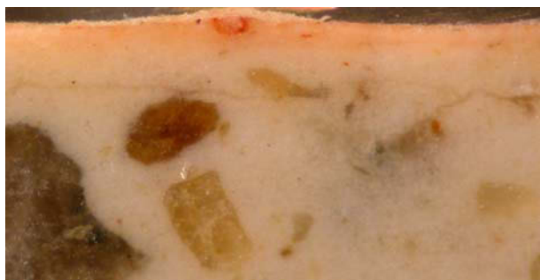
Figure 6: The presence of a lime-wash layer typical of murals at Zanigrad and Pomjan.
