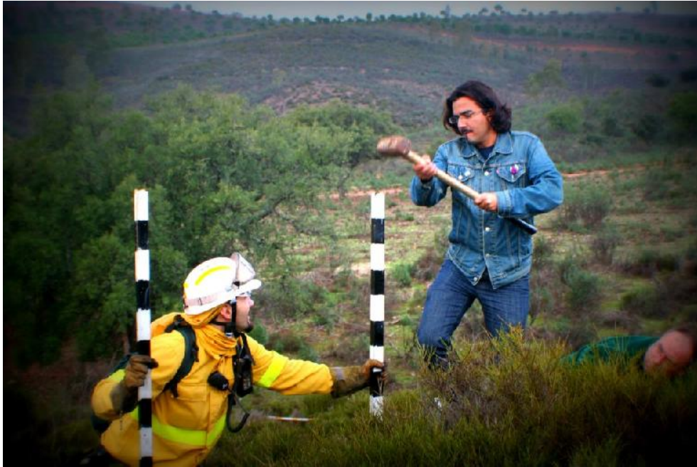
Figure 12: Installation of bars for determining flame height.
