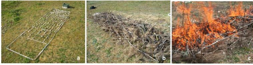
Figure 4: Some details of the experimental work: (a) soil plots with 0, 15, 30, 45 and 60% Stone cover; (b) soil plot after addition of fuel; (c) soil plot during burning.
