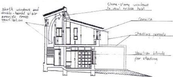
PASSIVE COOLING SYSTEM
