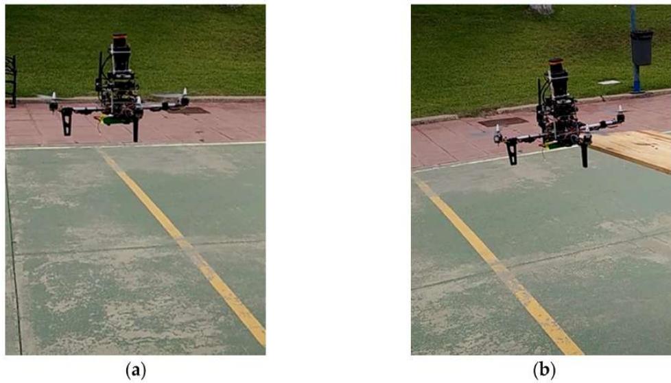
Figure 3.21: Partial ground effect tests with multirotor flying outdoors: a) multirotor in free flight; b) multirotor flying under partial ground effect (the rotor at the right with a ground plane close to it)
