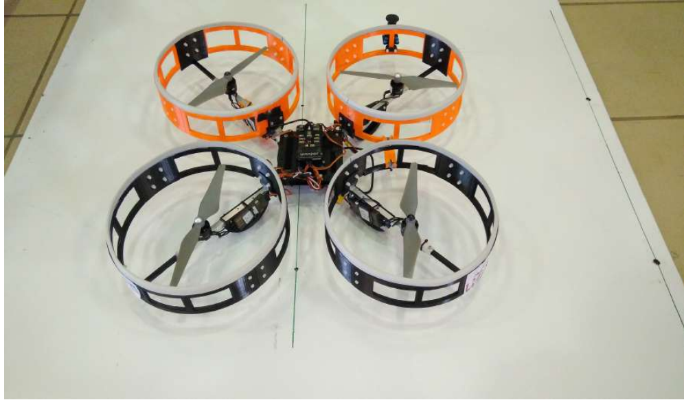
Figure 4.1: First prototype of the bridge inspection platform
