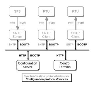
**Fig. 1.** Typical scenario for deploying hardware SNTP client and servers (synchronization devices and protocols are marked in gray, and configuration devices and protocols are marked in black).
