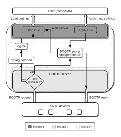
Fig. 3. Overall diagram of the configuration server operation.
