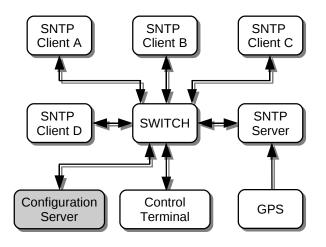
Fig. 4. Environment used to test the configuration server.
