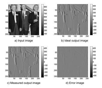
Fig. 13. Experimentally obtained convolution processing results with a kernel for vertical edge extraction of a  $256 \times 256$  input image. (a) Input image. (b) Ideal output image. (c) Measured output image. (d) Error image.
