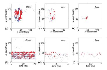
Fig. 2. Illustration of pseudosimultaneity when a ConvChip filters events produced by a motion sensitive retina. (a) ConvChip input (dots) and output (circles) events captured simultaneously during 40 ms, represented in the (x, y)coordinate plane. (b) Same events represented in the (x, time) plane. (c)–(d) Represent the same than (a-b) but for a subset of events during the first 4 ms, and (e)–(f) for the first 1 ms.
