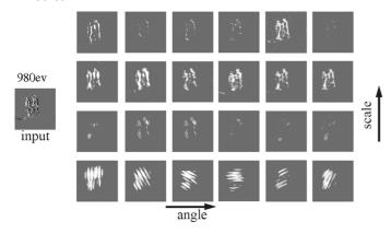
Fig. 3. Illustration of pseudosimultaneity for a  $6 \times 4$  array of Gabor filters of different scales and orientations. Input and output events correspond to the same 40 ms time window.
