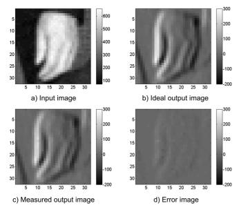
Fig. 11. Experimentally obtained convolution processing results with a kernel for vertical edge extraction. (a) Input image. (b) Ideal output image. (c) Measured output image. (d) Error image.
