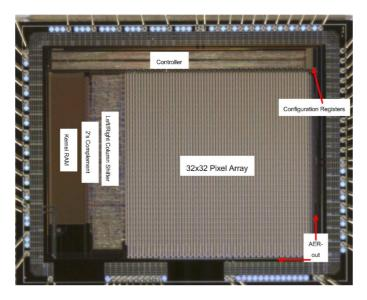
Fig. 7. Photograph of the fabricated  $32 \times 32$  pixel fully digital convolution chip.
