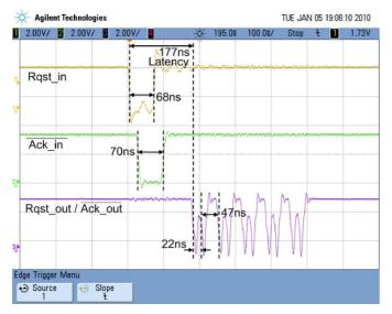
Fig. 8. Measured input and output events Rqst and Ack signals when maximum clock frequency is set to  $f_{clock} = 120$  MHz, with shorted  $Rqst_{out}$  and  $Ack_{out}$ . The oscilloscope used is Agilent DSO7054A, with a bandwidth of 500 MHz and a sample rate of 4 GSa/s.
