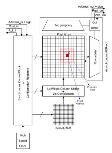
Fig. 4. Architecture of the convolution chip.
