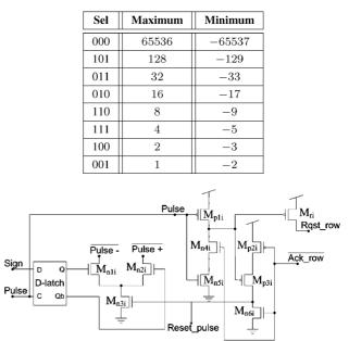
Fig. 6. Schematic of the interface block inside the pixel.
