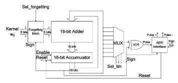
Fig. 5. Block diagram of the convolution pixel.
