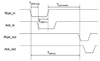
Fig. 9. Time delay between input and output events.
