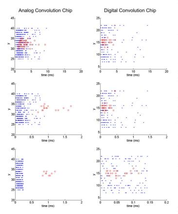
Fig. 17. Results for processing the circle of LEDs and discriminate the center, both with the analog convolution chip and the digital one. Dots represent the events generated by the retina, and circles represent the events generated by the convolution chip, being the y-axis the y-address of the events. Each row shows the results for different durations of the input burst.
