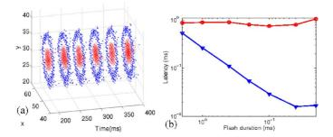
Fig. 16. (a) 3-D representation in (x, y, time) space of the 40 ms period ON and OFF retina transients (dots) and convolution chip outputs (circle) when exposed to a flashing circle of LEDs. (b) Measured latency between input and output events for different values of the LEDs flash duration; circles correspond to the analog chip, and triangles to the digital chip.
