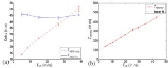
Fig. 10. (a) Measured values for  $T_{AER-chip}$  and  $T_{AER-Tx}$  for different settings of  $T_{clk}$ . (b) Measured values of  $T_{latency}$  for different settings of  $T_{clk}$ ; each measurement was repeated 5000 times and error bars indicate measured spread; dotted line represents linear fit ( $y = 8.2 \times x + 97$ ).
