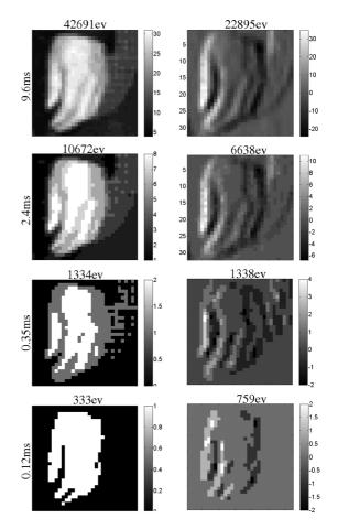
Fig. 12. Speed characterizations of convolution processing. Top row: input image pixels coded from 0 to 32 events with an event burst duration of 9.6 ms, convolution output is captured synchronously with the input during the same 9.6 ms. Second row: same as above, but capturing input and output events synchronously during the first 2.4 ms only. Third row: same, but during the first 0.35 ms. Fourth row: same, but during the first 0.12 ms.
