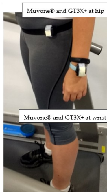
Figure 1. Muvone® and GT3X+ accelerometers adjacent and taped together, positioned over the non-dominant hip and wrist.
