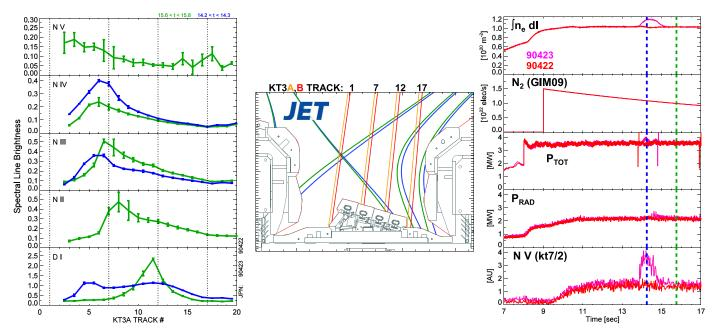
Fig. 7. Example of enhanced spectroscopic tools used in JET L-mode experiments. Spatial profiles of D I and N II-V (left) are shown for chords viewing across the outer divertor (middle) at two different time points in repeated discharges that employed a weak strike point scan (right).
