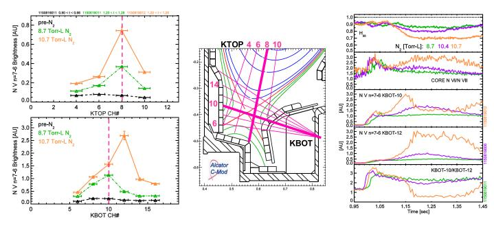
**Fig. 8.** Example of spectroscopic methods implemented at Alcator C-Mod where spatial profiles of N V n = 7-6 emission in the divertor are tracked as private flux nitrogen fueling is increased shot-to-shot. Movement of emission layers is shown to follow confinement degradation.
