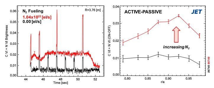
Fig. 6. Demonstration of active and passive N VI charge exchange showing enhancement during NBI (left) and the transition from C VI dominated to mixed N VI and C VI emission profile (right).
