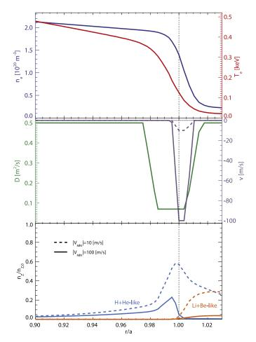
**Fig. 3.** (top) STRAHL input  $T_e$  and  $n_e$  profiles with (middle) diffusion and convection profiles estimated to model an edge transport barrier. A limited range of charge state density profiles (bottom) are plotted for two possible peak convection values.
