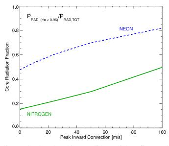
**Fig. 4.** Resulting change in spatial structure of the 1D radiation profile computed from STRAHL simulations, showing an inward shift of radiation as convection is decreased to -100 m/s.
