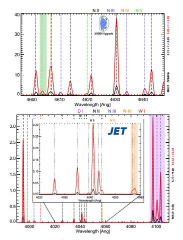
**Fig. 5.** Measured spectra from boundary plasma showing ranges to observe N V (top) and N II-IV (bottom). High resolution is required to avoid overlap with D I and N II lines for N III, N IV and N V. Note that spectra are plotted versus angstroms while line positions are given in nanometers in the next.
