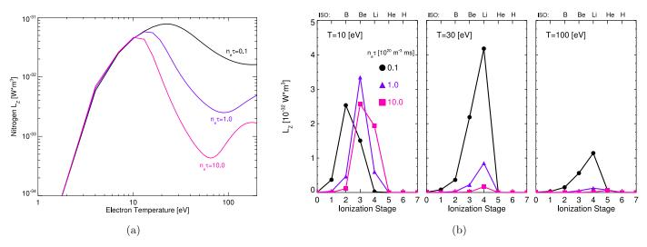
**Fig. 2.** (a) Demonstration of the enhancement of nitrogen radiation for ions out of ionization equilibrium, showing a large increase in  $L_Z$  as  $n_e \tau$  is reduced and (b) how this enhanced radiation is distributed among different ionization stages.
