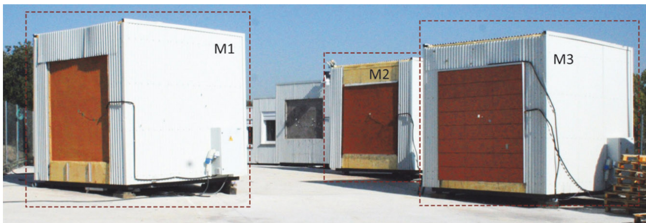
Figura 3. View of south façade on the three GESLAB test cells.
