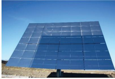
Fig. 7. Photograph of shadowed heliostat. CTAER Tabernas, Almería.
