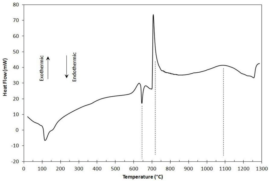
Fig. 7. DSC curve of the as-blended mixture in the Mg/ $\text{ZrSiO}_4$ / $\text{B}_2\text{O}_3$ /C system.
