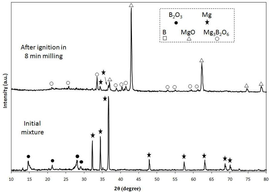
Fig. 5. X-ray diffraction patterns of the initial and milled samples of the Mg/B<sub>2</sub>O<sub>3</sub> system.
