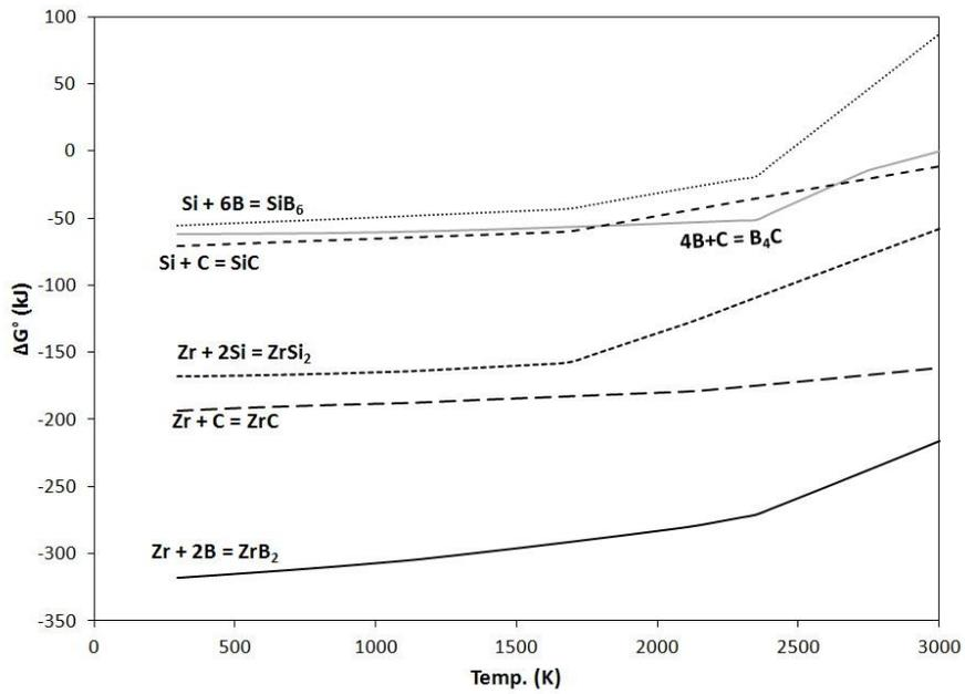
Fig. 4. Standard free energy of formation for various potential compounds capable of being created from elemental Zr, Si, B and C.
