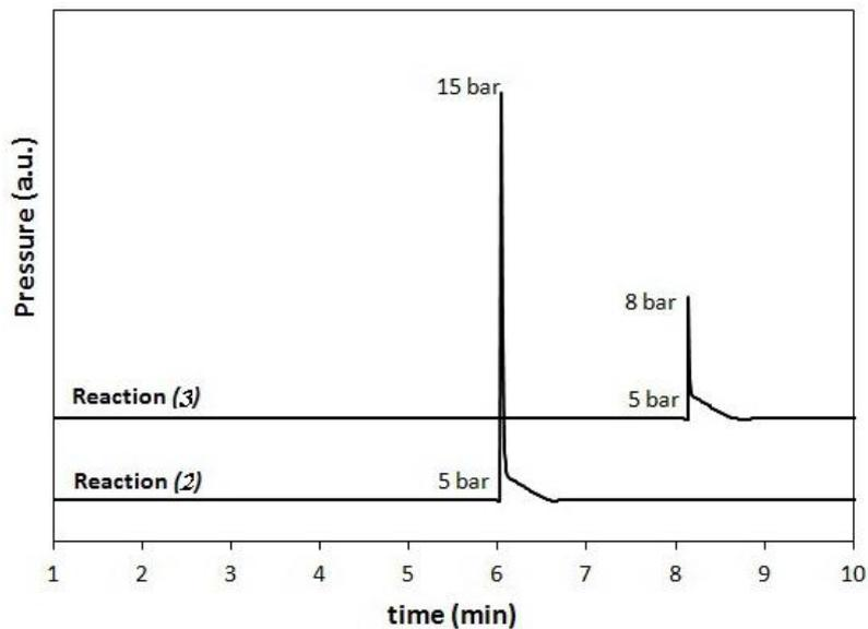
Fig. 1. Pressure inside the vial versus milling time for the Mg/ZrSiO<sub>4</sub>/B<sub>2</sub>O<sub>3</sub>/C (reaction 2) and Mg/B<sub>2</sub>O<sub>3</sub> (reaction 3) systems.
