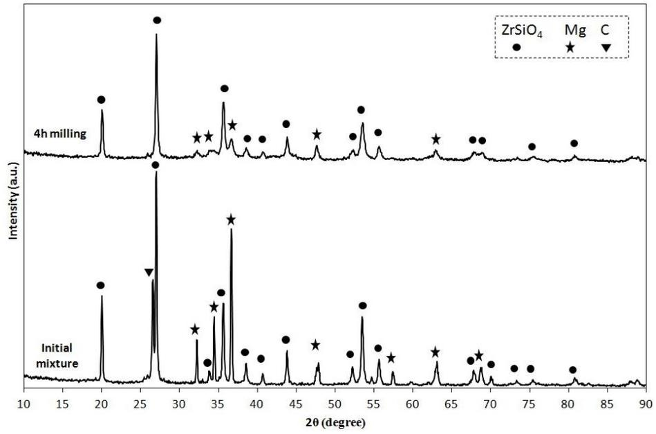
Fig. 6. X-ray diffraction patterns of the initial and milled samples of the Mg/ $\text{ZrSiO}_4$ /C system.
