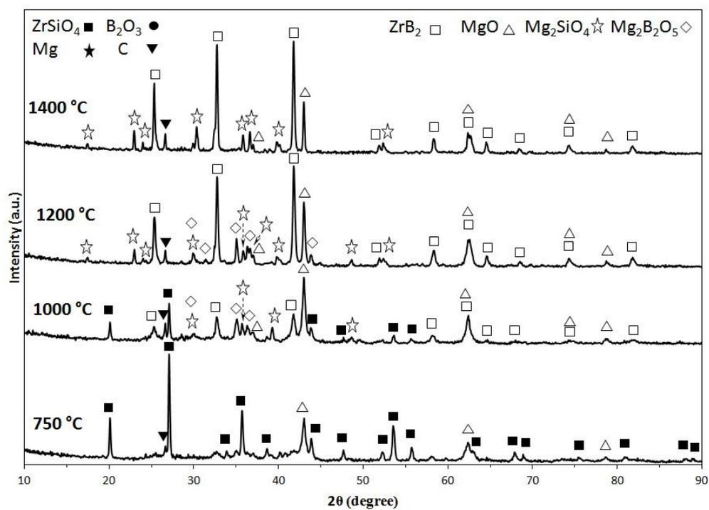
Fig. 8. X-ray diffraction patterns of the blended powders in the Mg/ZrSiO<sub>4</sub>/B<sub>2</sub>O<sub>3</sub>/C system after heating at 750, 1000, 1200 and 1400 °C (30 min dwell time at maximum temperature prior to cooling inside the furnace to room temperature).
