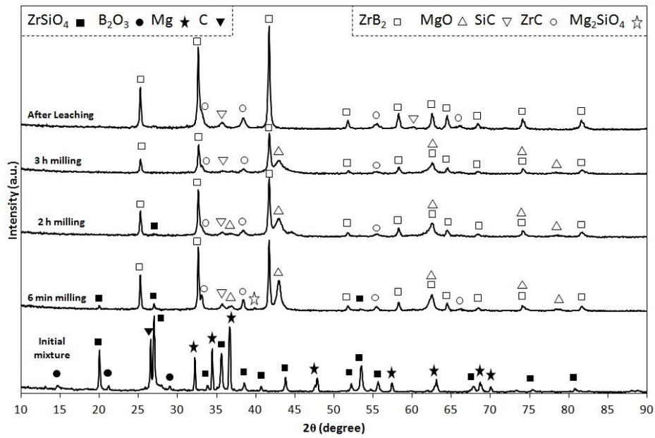
Fig. 2. X-ray diffraction patterns of the as-blended, milled and leached samples of the Mg/ZrSiO<sub>4</sub>/B<sub>2</sub>O<sub>3</sub>/C system.
