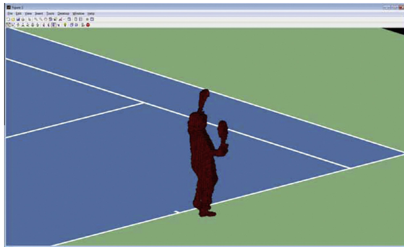
Fig. 3. An example of the output of the voxel carving technique when applied to one frame from a tennis match dataset (3DLife ACM Multimedia Grand Challenge 2010 Dataset) [14].
