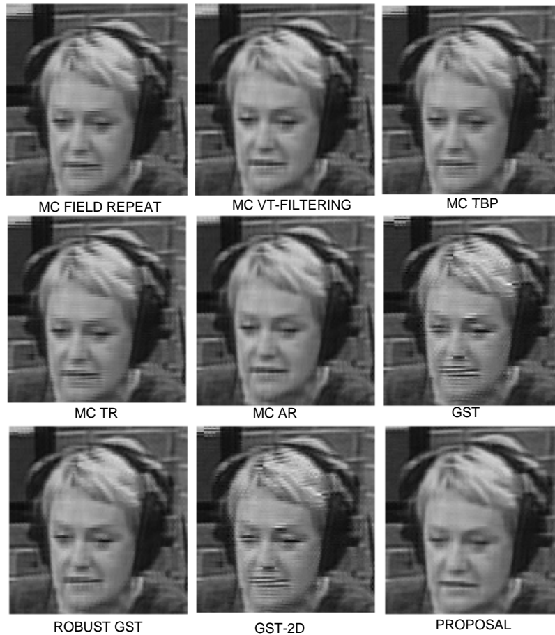
Fig. 15. Deinterlaced images obtained with MC de-interlacing algorithms and our proposal in the Donna hybrid sequence (film area).
