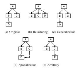
Figure 12: Types of relationships between two feature models
