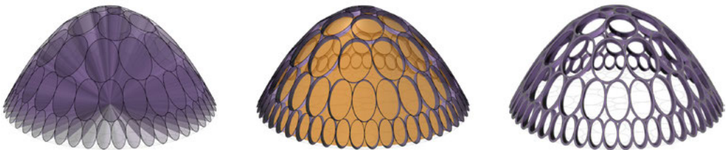
Figure 3. Left: Discretisation of the dome with elliptical rings and generation of the cones by extruding the ellipses to the centre of the base of the dome. Middle: Offset surface to trim the apex. Right: Thickening of the conical rings as an immediate solution to acquire rigidity.
