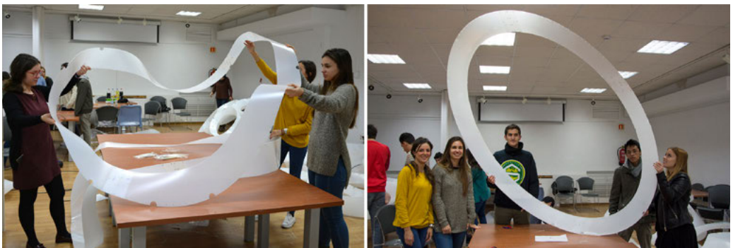
Figure 5. Left: Photograph of the unrolled conical surfaces before assembly. Right: Result of the conical component after assembly and the emergence of the desired structural rigidity.
