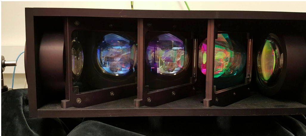
Figure 2: Top: the Zemax design of the Barcelona LIDAR polychromator. Bottom: A picture of the polychromator taken from the bottom side.
