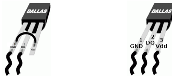
Illustration 4. Parasite and normal mode of DS18B20 sensor. [1]
