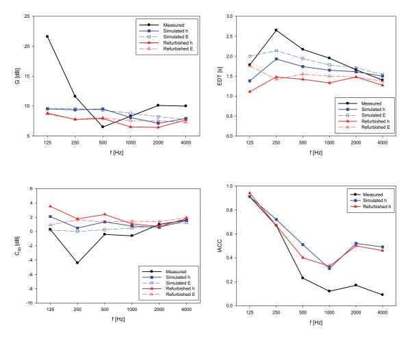
**Figure 16**. Measured -in black- and simulated -in blue and red, regarding before and after refurbish- data for some room acoustics parameters at receiver A-1. From top to bottom, and left to right: sound strength (G), early decay time (EDT), clarity ( $C_{80}$ ), and interaural cross-correlation coefficient (IACC). For the sake of comparison, simulated values from energetic analysis (E) –in contrast to those from IRs (h)- are depicted with dashed trace.
