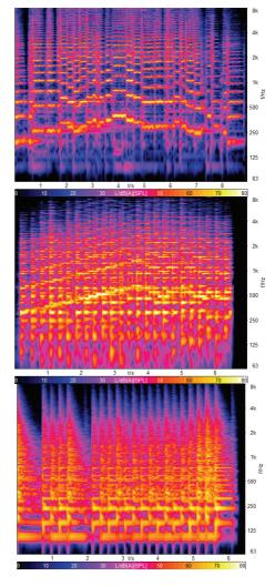
**Figure 15**. Frequency spectra (FFT) versus time for A-weighed sound pressure level (SPL) in dBA of the original fragments of anechoic recordings auralized for the experiments. From top to bottom: cello, piano and timbales sample spectrograms.
