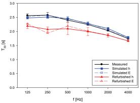
**Figure 18.** Spatially-averaged reverberation time  $(T_{30})$  assessed at the three receivers in this work. Measured –in black- and simulated records –distinctively using blue and red colours for before- and after-refurbish states- are shown. Energy (E) and pressure analyses (h) have been also differentiated by dashed plot for the latter.
