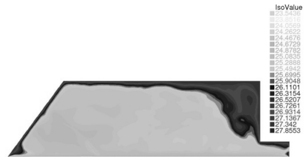
Figure 6: Energy simulation using CFD. Room with mur neutralisant and respiration exacte studied for a summer day.
