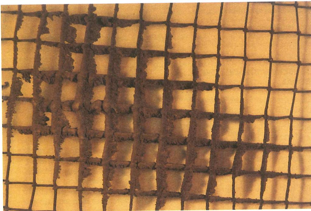
Figure 3 Precipitated deposit on a grille placed in 1948.
