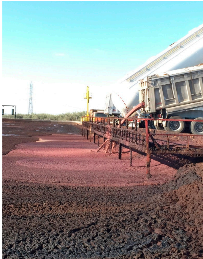
Figure 7. Olive pomace from oil mills that use the centrifugation process with a two-outlet decanter. These pomace rafts are located in the extraction plants of pomace oils.
