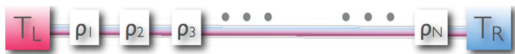
FIG. 1. (Color online) The model is defined on lattice sites, each one characterized by an energy \rho_i . The dynamics is stochastic and proceeds via random collisions between nearest neighbors where part of the pair energy is dissipated to the environment and the rest is randomly redistributed within the pair. Such dynamics mimics at the mesoscopic level the evolution of a wide class of systems characterized by a nontrivial competition between diffusion and dissipation.
