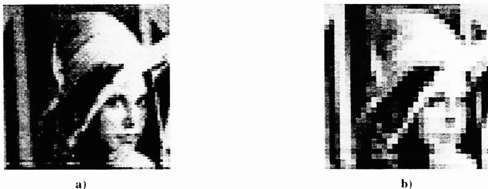
Figure 6. (a) Full resolution ( 64 \times 64 ) image taken at 5MHz read-out rate. (b) Same image taken at 32 \times 32 pixels resolution. Integration time in both cases is 1.4ms
