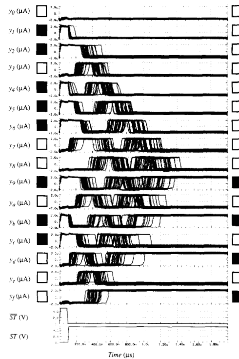
Fig. 21. Monte Carlo results for the CT full range CCD prototype.
