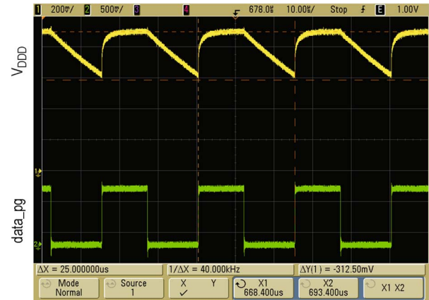
Fig. 16. Measured signals in the experimental setup of Fig. 15(a). Input signal data\_pg is a 40-kHz pulse train with 1-V amplitude and 47.5% duty cycle. The peak amplitude of the rectified signal V_{DD} is 0.9 V, and the voltage drop is 312.5 mV.
